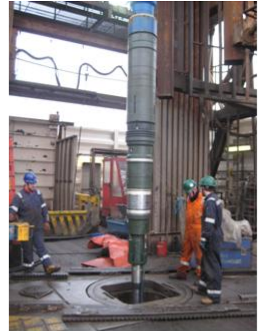
Tubing Hanger with optical fiber feed through system running in hole
